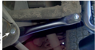
Rear brace arrangement passenger side looking back
